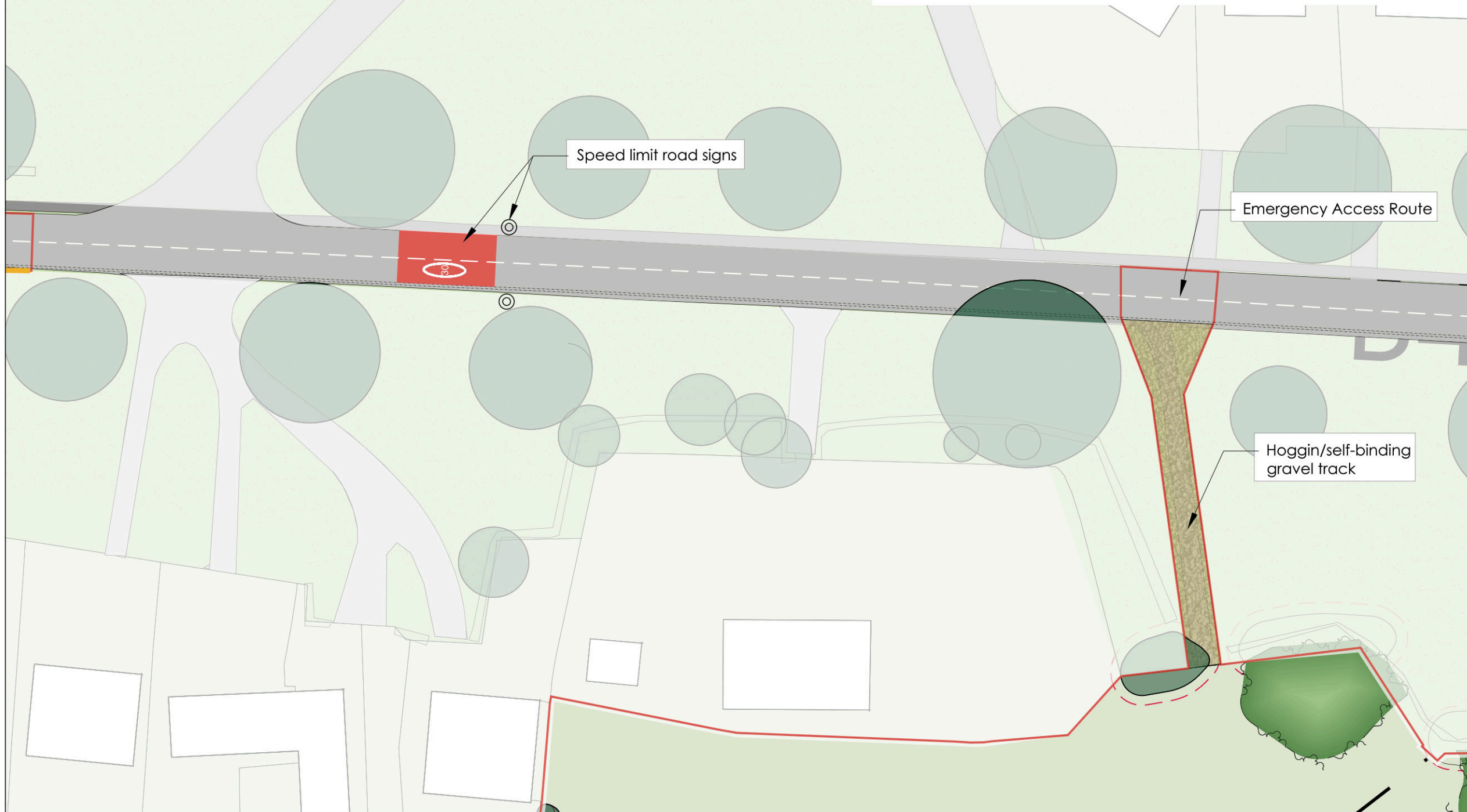
Hoggin surface: Compacted, fine-screened 'hoggin' surfacing, nominal 50mm compacted layer over min. 150mm Doft Type 1 sub-base; softwood timber edging, pegged in place.
