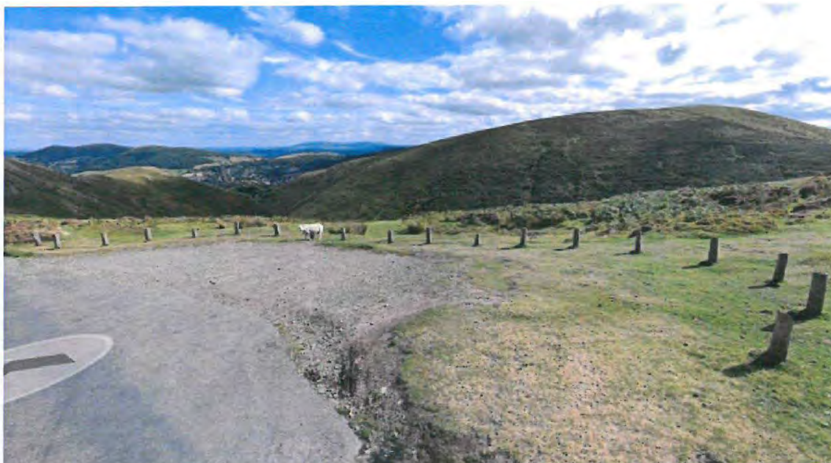
Stobs in use at Carding Mill Valley, AONB. National Trust. Spec: wooden, slanted top, round, 30cm high, no reflective markers, unpainted.
